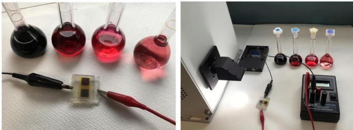
Figure 13. A Dye Sensitized Solar Cells prototype, assembled by valorizing winemaking waste, tested under simulated solar light irradiation.
