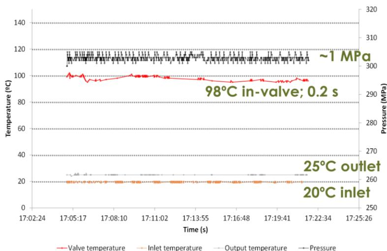
Fig 3. Thermal and pressure conditions during the in-valve flow (adapted from complementary material published in Loira et al, 2018).
