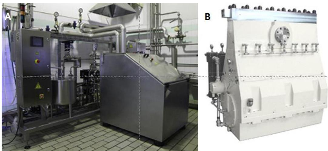
Fig 1. 200-400 MPa continuous technology Ypsicon(A). UHPH pump 10,000 l/h (B).
