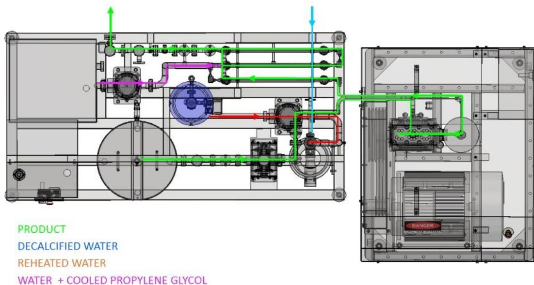
Fig 2. UHPH system section showing the product flow.
