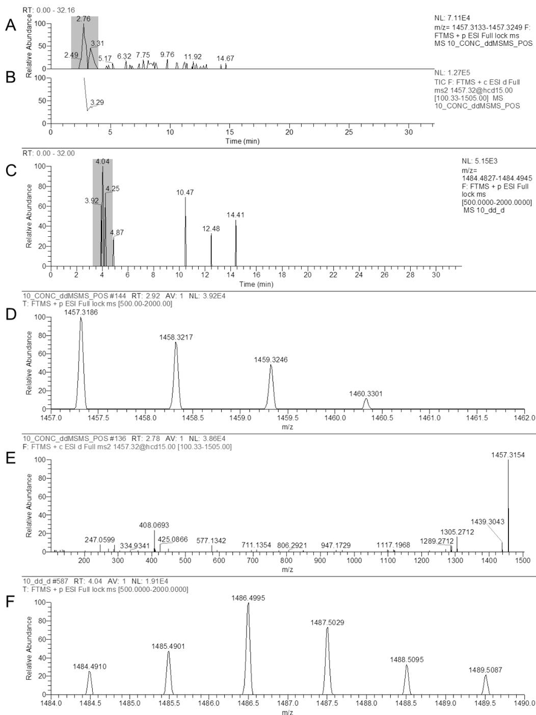
Figure 3. *c-pentamer-1-galloyl* (R.t. = 2.8 min). A) EIC(H); B) TIC(H) of MS/MS; C) EIC(D); D) HRMS(H) at 2.9 min; E) MS/MS(H) spectrum at 2.8 min; F) HRMS(D) at 4.0 min. The parts highlighted in green show the peak associated with the identified cyclic oligomers.
