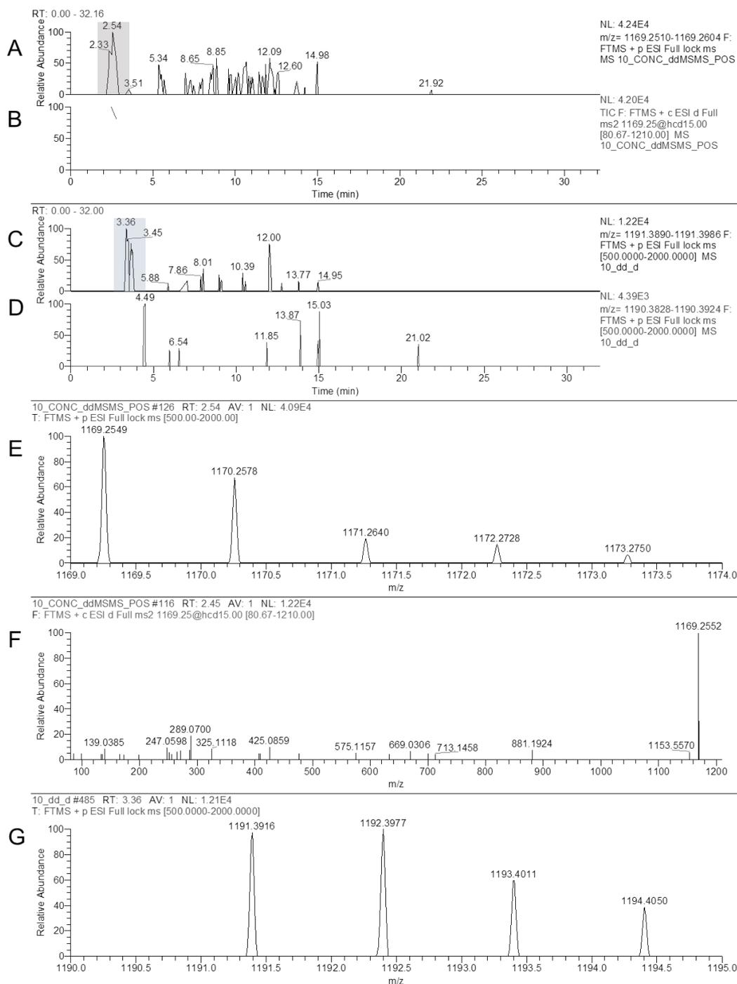
Figure 2. *c*-tetramer-1-gallic (R.t. = 2.5 min). A) EIC{H}; B) TIC{H} of performed MS/MS analysis; C) EIC{D}; D) EIC{D} of 1190.3876 m/z (corresponding to the isomeric *a*-tetramer-1-gallic); E) HRMS(H)
