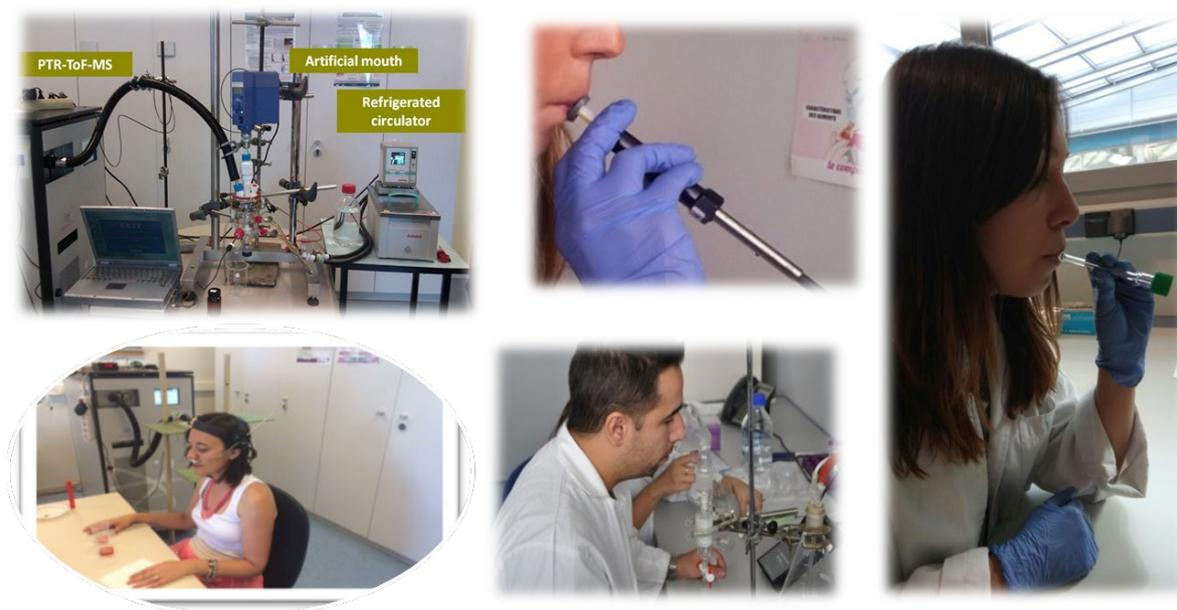
Figure 1. Different methodologies for aroma analysis during wine consumption. (a) artificial-mouth-PTR-ToF-MS; (b) intra-oral SPME-GCMS; (c) in-nose PTR-ToF-MS; (d) RATD-CIS-GCMS; (e) in-mouth-HSSE-TDU-GCMS
