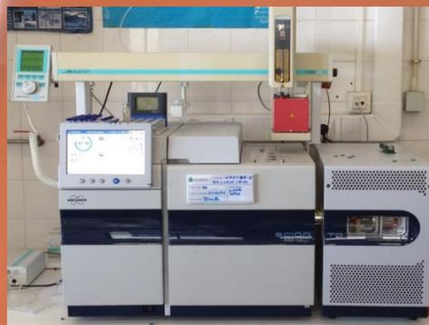
Analytical columns: ZB-WAX PLUS (30 m x 0.25 mm i.d., 0.25 µm df) connected with a ZB-5 MS (30 m x 0.25 mm i.d., 0.25 µm film df).
