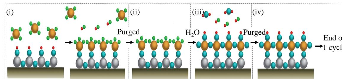
Figure 1. Sequence of zirconium oxide deposition on alumina surface by ALD
