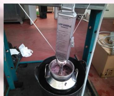
*Img. 1.* Ultrasound vinification system
