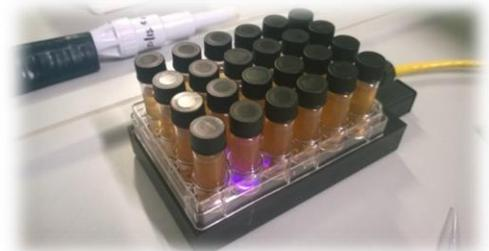
Sensor dish reader used for the study of must oxygen consumption
