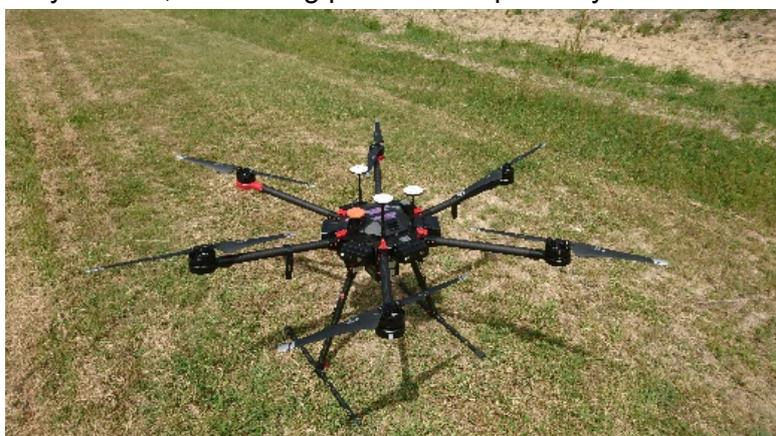
Figure 1. The UAV used by VineView for vegetation mapping
