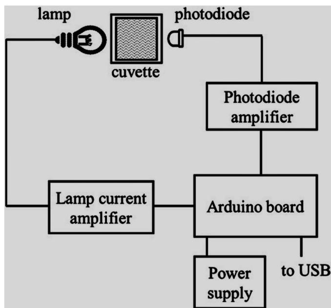
**Figure 1.** Schematic representation of the optical device described in Ragni et al., 2016 as reported in Ricci et al., 2020.
