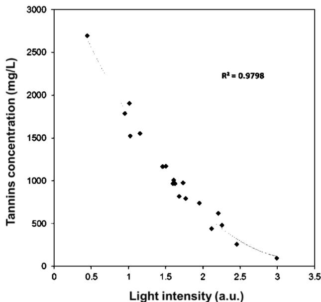
**Figure 2.** Non-linear correlation between the tannin content in wines and the peak light intensity as measured following the mixture of wine with gelatin solution and development of turbidity.
