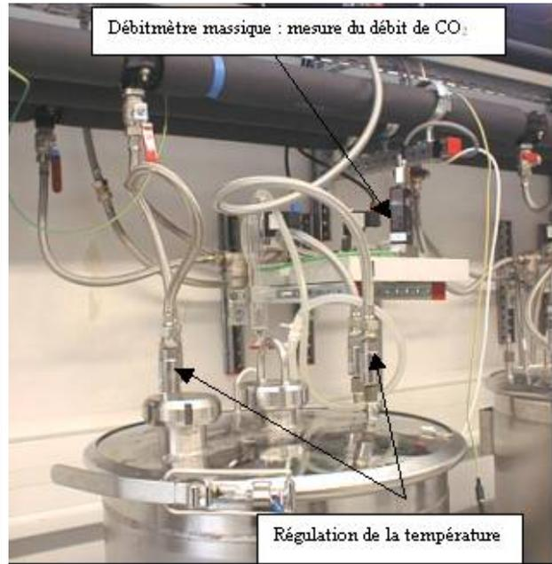
Picture 2: detail of tank head plate
