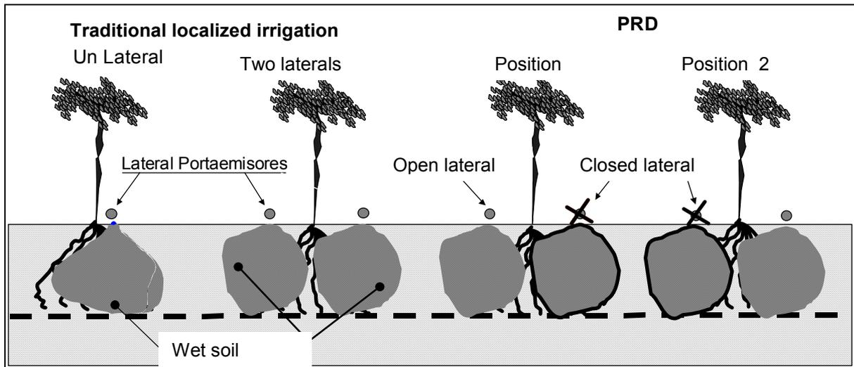
Figure 1. Illustration of traditional and PRD localized irrigation systems.
