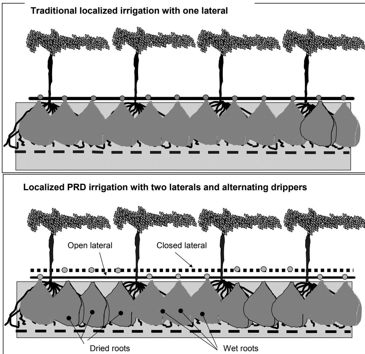
Figure 3. Localized irrigation systems A) traditional with one lateral; B) PRD with two laterals and alternating drippers between the vines.
