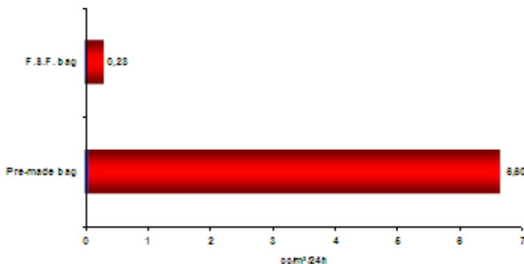
Figure 4. An Oxygen Transmission Rate Comparison between a Form-Seal-Fill and Pre-Made Bag made with the same Film
