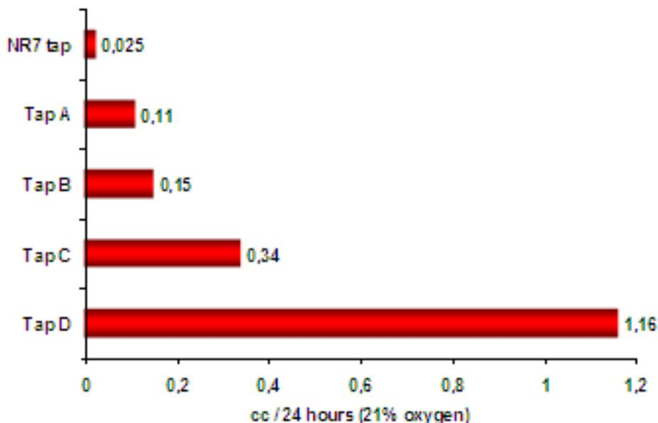
Figure 5. An Oxygen Transmission Rate Comparison between Flexainers' NR-7 and other Popular Wine Taps
