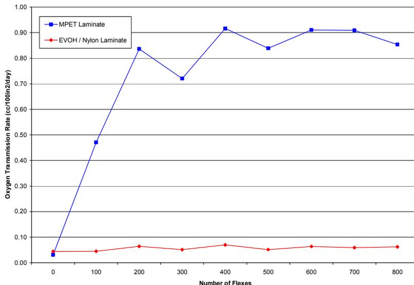
Figure 3. The Relationship between Oxygen Transmission Rate and Number of Flexes for MPET and EVOH / Nylon Laminates
