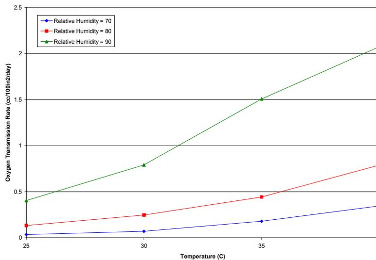
Figure 2. The Relationship between Oxygen Transmission Rate, Temperature, and Relative Humidity for Standard EVOH
