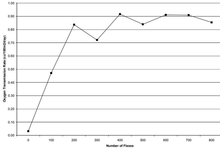
Figure 1. The Relationship between Oxygen Transmission Rate and Number of Flexes for MPET
