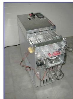
Figure 1. HIPEF equipment OSU 4F used in this study for must treatment.
