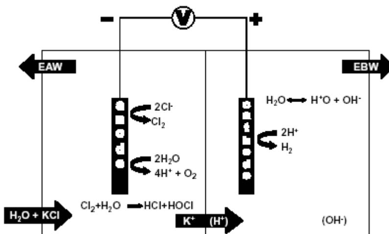
Fig. 1. The system for producing EAW and EBW
