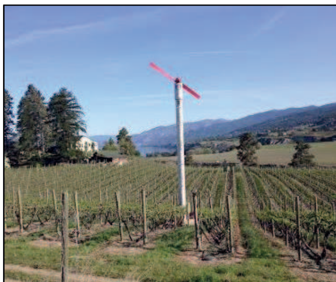
Fig. 1: Wind machines reduce freeze damage by drawing down warm air from several metres above grapevine canopies to mix with cold air near the ground.
